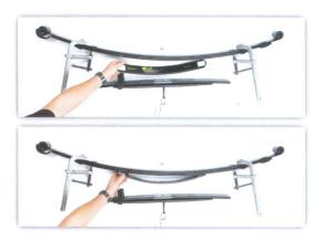
**4.** Gently tap the new centre bolt through the springs being careful not to damage the thread. Install the nut and tighten until moderate tension is felt.
